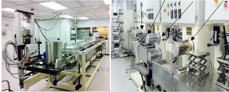
Figure A.1 Multifilament fiber spinning (left) and multistage drawing facility (right).
