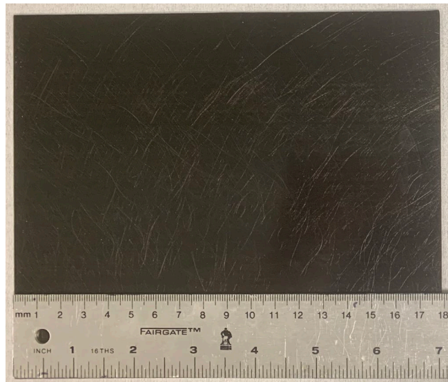
Figure B.3 6-ply unidirectional hollow CF composite panel manufactured at University of Southern Mississippi. The panel shows significantly higher number of misaligned fibers compared to the IM7 composite panel. This is due to the higher number of broken fibers in the hollow CF tow compares to the commercially produced IM7 fiber tow.
