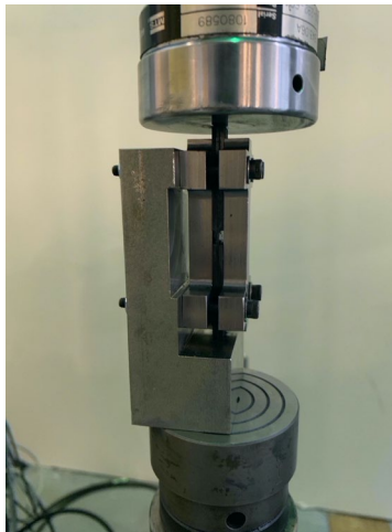
Figure 3.2 Specimen support fixture for modified ASTM D695 compression test
