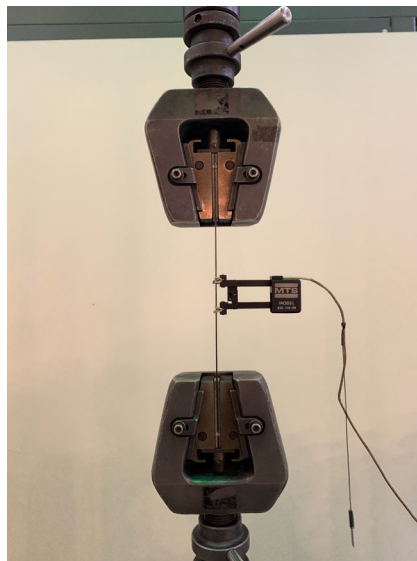
Figure 3.1 Composite specimen with extensometer mounted for ASTM D3039 tension test
