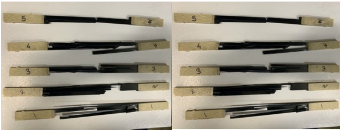
Figure B.7 Failed IM7 composite specimen under tension at room temperature (left) and -75°F (right). The failure mode per ASTM D3039 can be characterized as split-gauge length – middle (SGM) for both temperatures.
