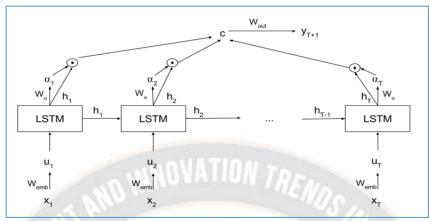
Figure 3: RNN (LSTM) with hidden states having linear and non-linear models
