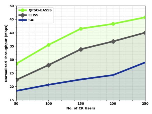
Fig. 3. NTHR analysis of QPSO-EASSS system with varying CR users
