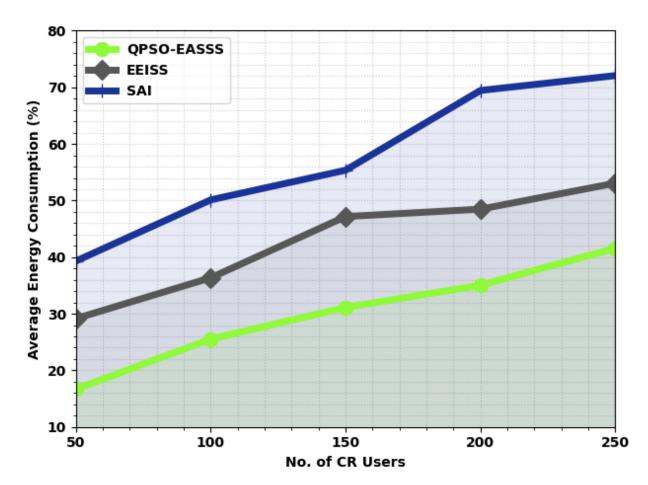
Fig. 6. AECON analysis of QPSO-EASSS system with varying CR users
