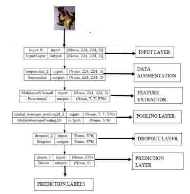
Figure 4: Model used for feature extraction and prediction.
