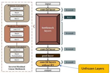
Figure 6: MobileNetV3 architecture (Qian et al. 2021) and the position of unfrozen layers.
