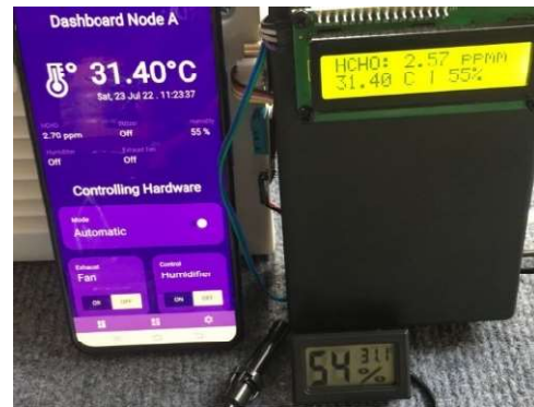
Figure 10. Temperature sensor testing
