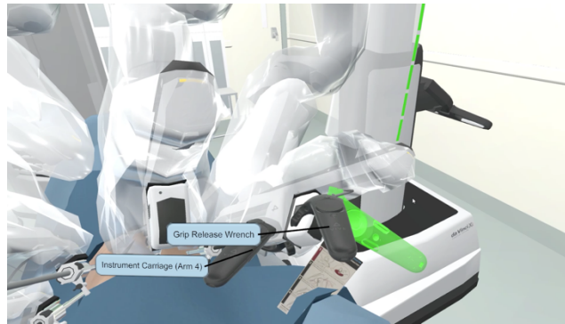
Figure A.4: Example of using the simple virtual hand technique to rotate the grip release wrench.
