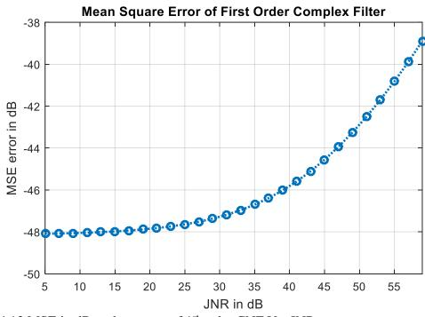
Figure 4.13 MSE in dB at the output of 1<sup>st</sup> order CNF Vs. JNR
