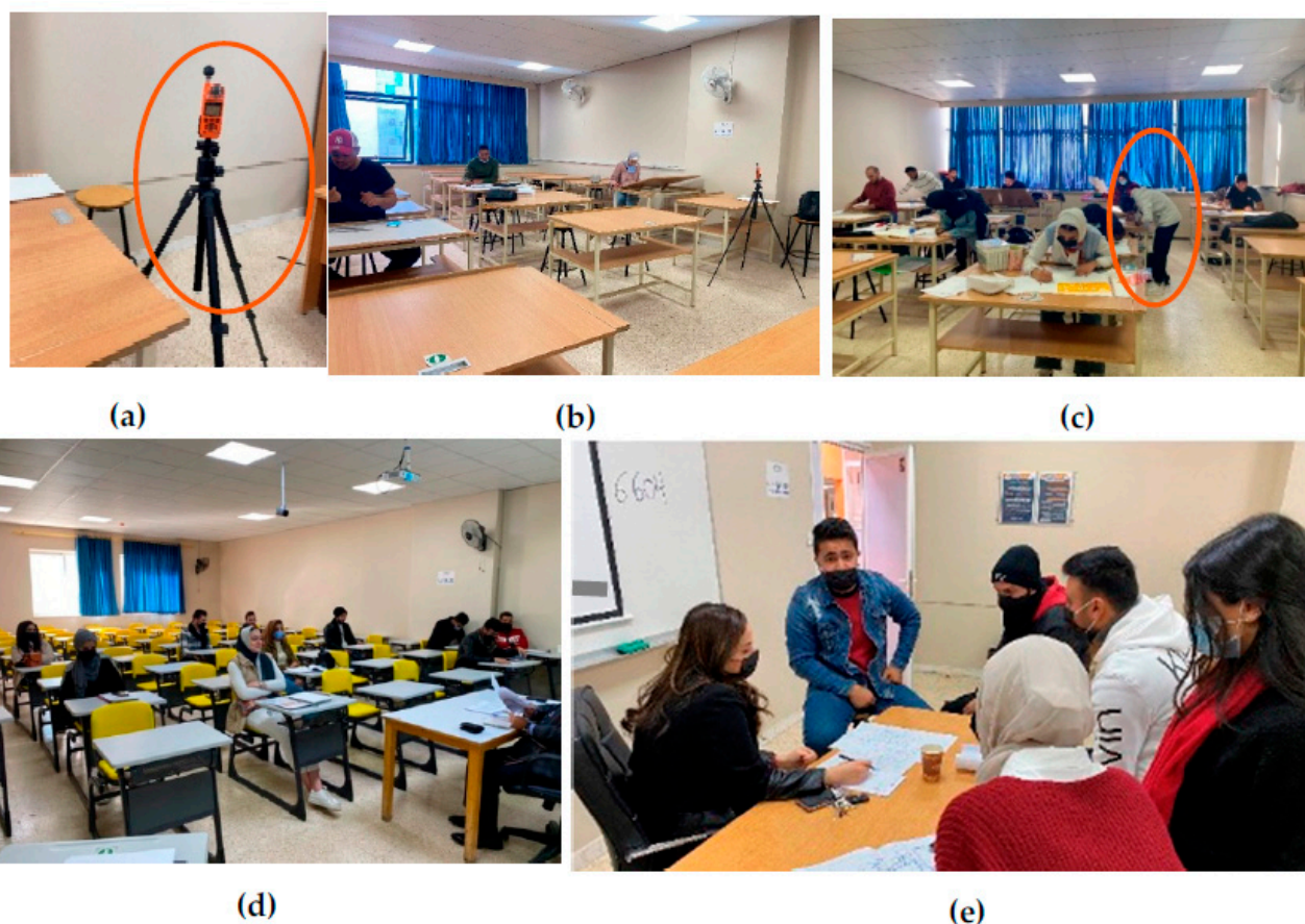
Figure 3. (a) The Kestrel Meter 5400 instrument; (b) the data logger positioned close to the students' desks; (c) students standing activities in architecture design studios; (d) students sitting with passive learning activities in the typical lecture room; (e) an example of focus group discussion done during the data collection stage.
