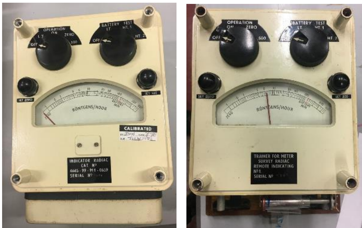
Fig. 3.3: Fixed Survey Meter (EF.1992.95.24) and the almost identical FSM Trainer (EF.1992.95.35), ©Sarah Harper.
