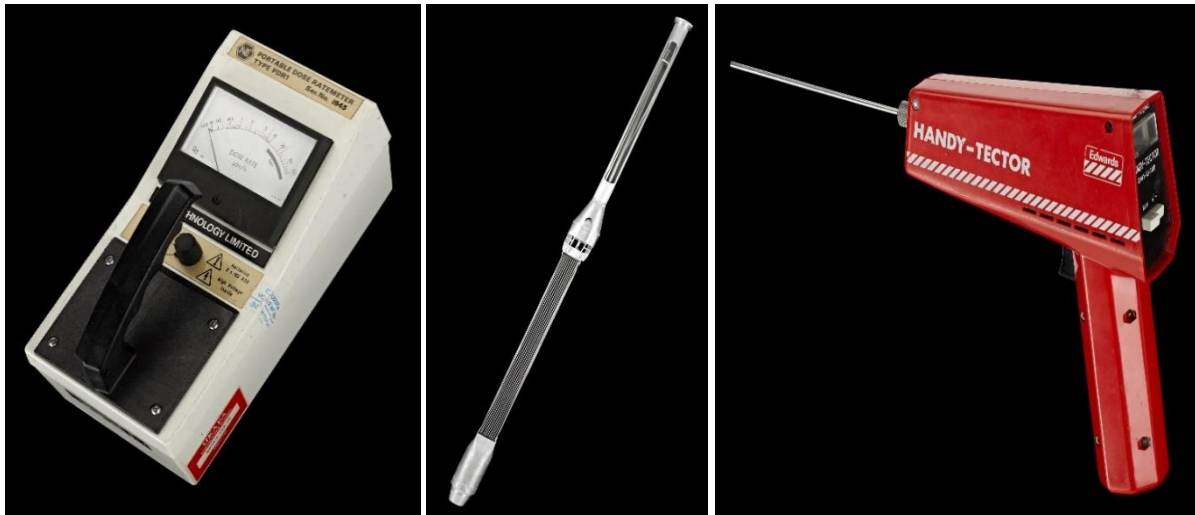
Fig. 2.1: Items donated by Dounreay Site Restoration Limited including a dose rate meter (T.2011.213), a materials testing reactor element (T.2011.203) and a helium detector (T.2011.220) ©National Museums Scotland.
