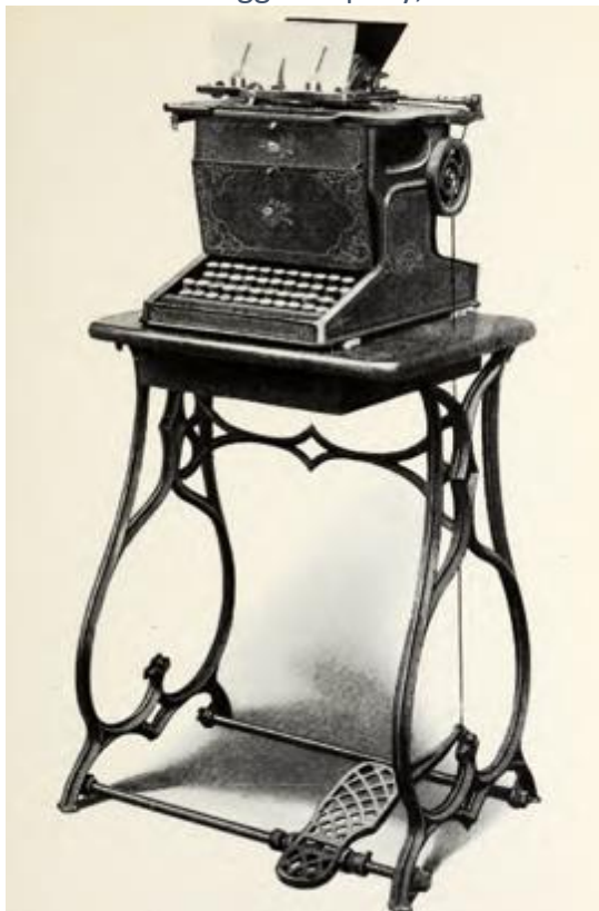
Figure 4.6. Sholes & Glidden manufactured by E. Remington & Sons c. 1874 with treadle for carriage return.
