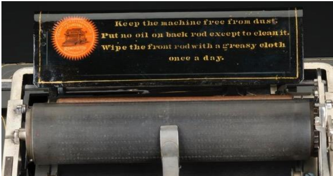
Figure 6.11. Paper feed for Remington Standard No. 2 typewriter, manufactured in 1887. NMS collection, object number T.1960.34.1.
