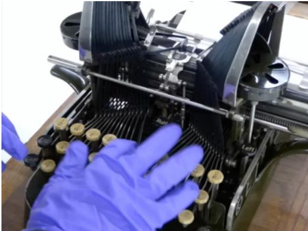
Figure 4.29. Oliver No. 3 typewriter with U-Shape typebars striking down onto the printing point. NMS collection, object number T.1959.39.
