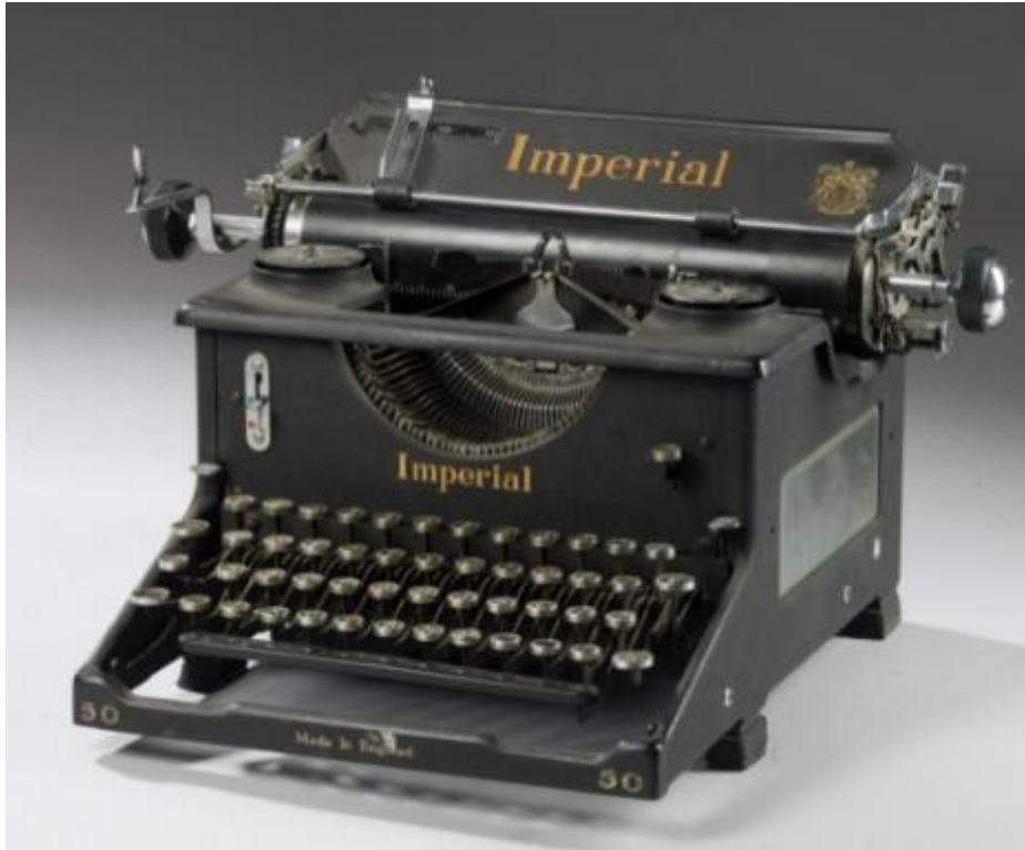
Figure 4.42. Imperial No. 50, which was strikingly similar in design to the Royal, even down to the glass panels on the sides. NMS collection, object number T.1988.88.
