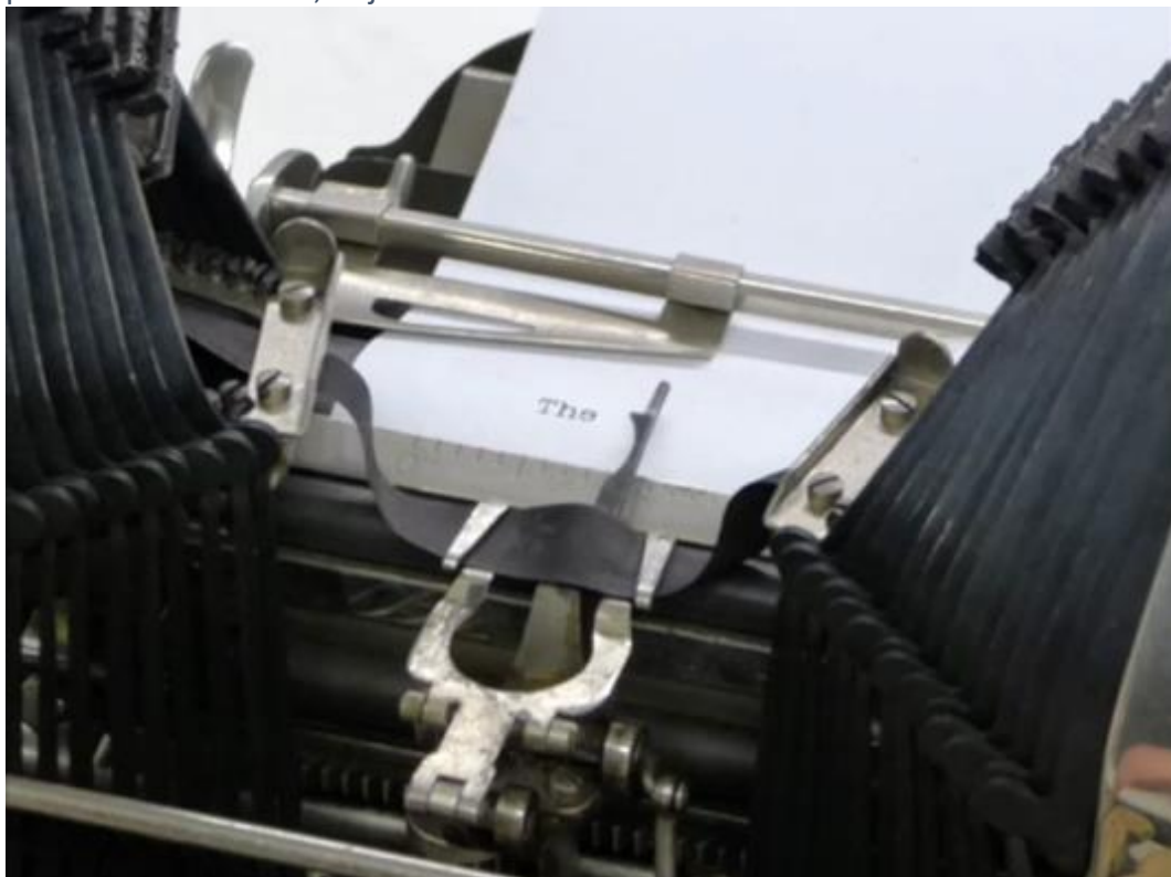
Figure 4.30. Close up of the Oliver showing the operator's line of sight to the text, which is blocked to the left and right.
