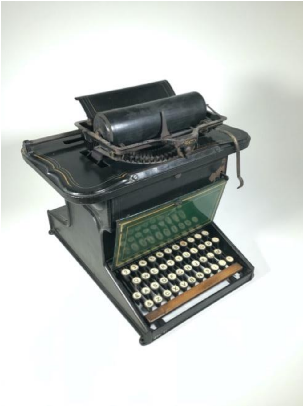
Figure 4.9. 'Perfected' Sholes & Glidden manufactured c. 1878, with a plain exterior and front lever for carriage return. NMS collection, object number T.1939.21.
