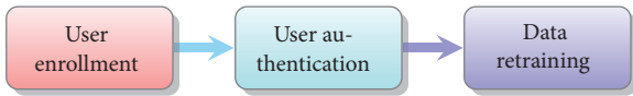
FIGURE 4: An authentication and authorization scheme using touch dynamics for mobile IoT devices. In the first phase, the touch dynamics data are acquired, processed, and stored. In the second phase, the system determines the similarity or dissimilarity. In the third phase, the reference template is updated (data adaptation).
