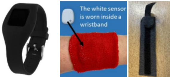
Figure 1: Three sensor-embedded wristbands (left to right): rubber strap, cotton sweatband, felt band.
