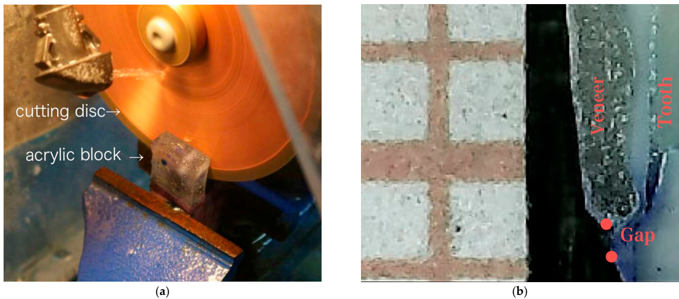
Figure 4. (a) Sectioning using Microtome cutter (b) Vertical section of veneer demonstrating marginal fit at the cervical region.
