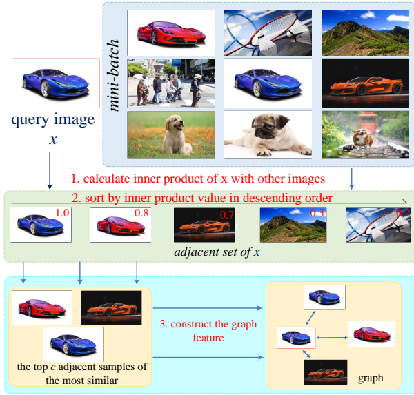
Fig. 4. Adaptive Computing to construct graph feature, taking the image modality as an example.
