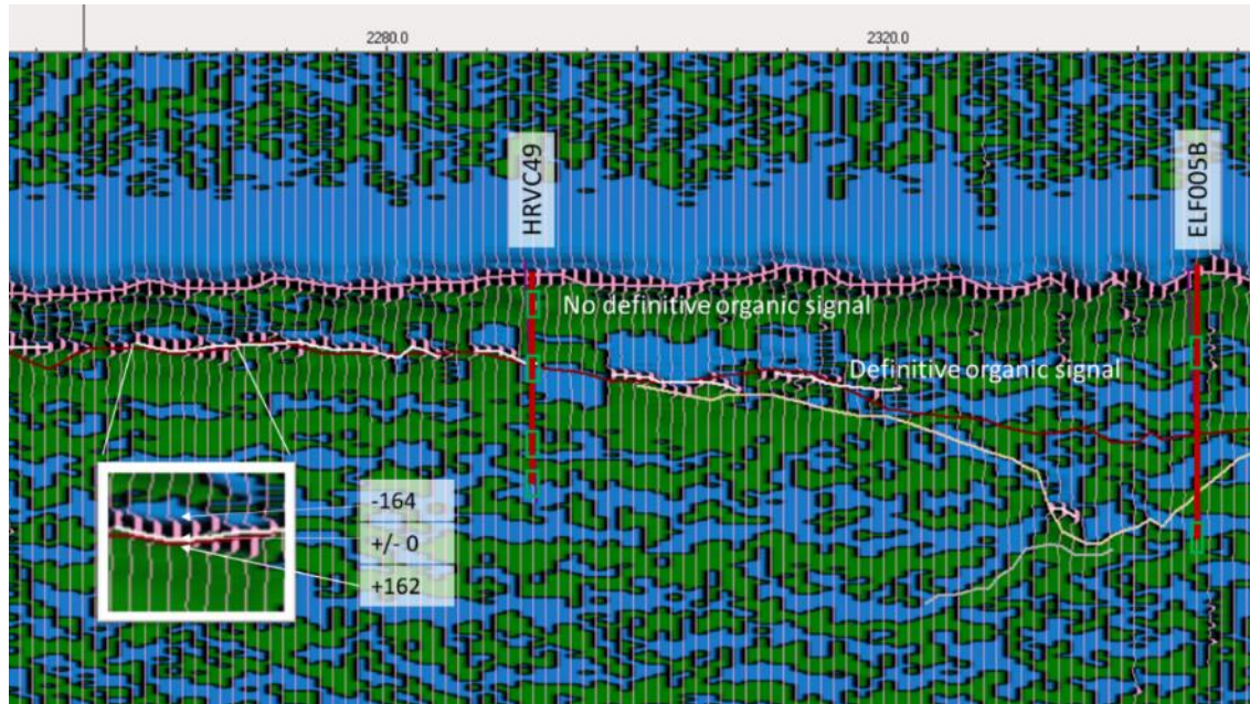
Figure 6.22 Phase Function shows very strong defined polarity between negative (blue) and positive and the zero charge variance peaks
