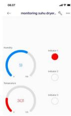
Figure 8 Display of Blynk Application Monitoring
