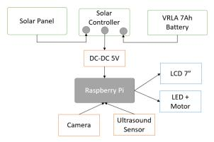
Figure 7. Hardware Connection of Monitoring System
