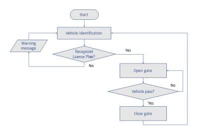
Figure 6. Working Diagram of Monitoring System
