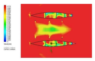
Fig. 13 - Cut-plot at current velocity 0.5m/s
