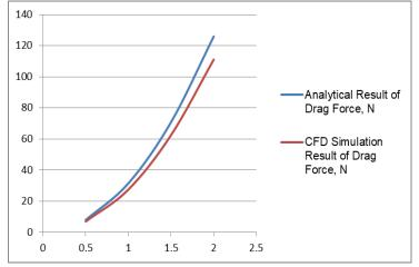
Fig. 10 - Analytical (vs) CFD simulation result drag force comparison
