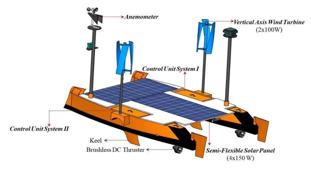
Fig. 6 - Mechanical 3-d hull structure design module connection in testing platform
