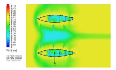
Fig. 12 - Cut-lot at current velocity 0.5m/s
