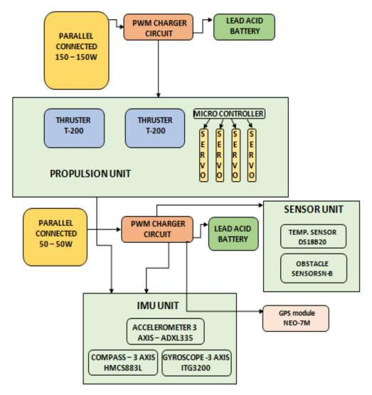
Fig. 1 - Autonomous smart ocean surface vehicles system
