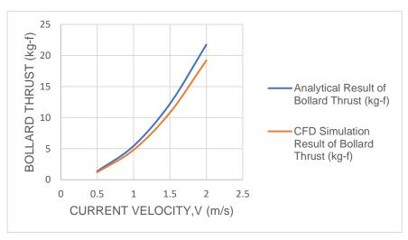
Fig. 11 - Analytical (vs) CFD simulation result bollard thrust comparison
