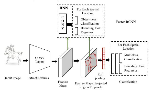
Fig. 5 - Faster R-CNN with RPN architecture
