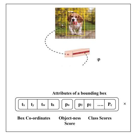
Fig. 11 - YoLo output format
