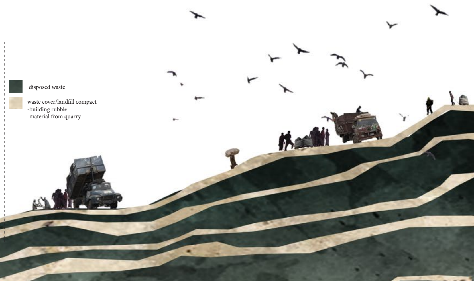
Figure 3.13: The Mechanics of the Landfill - a depiction of the layering system involved to create the accessible and dynamic landscape. Source: Author (2020)
