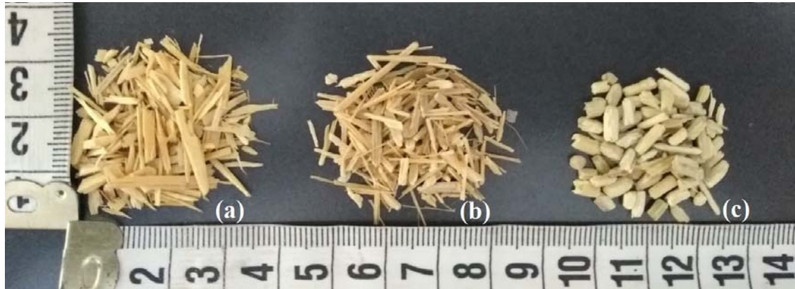
Figure 2: Particles commercial Pinus taeda (a), Bamboo (b) and Mate (c) produced in 144 the laboratory.
