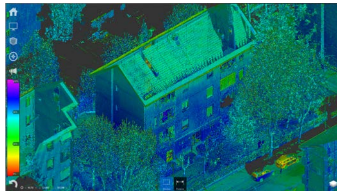
Fig. 4: Rilevo dell'esistente attraverso Scanner Laser 3d Fig. 4: Geometrical survey by means of Laser scanner 3d
