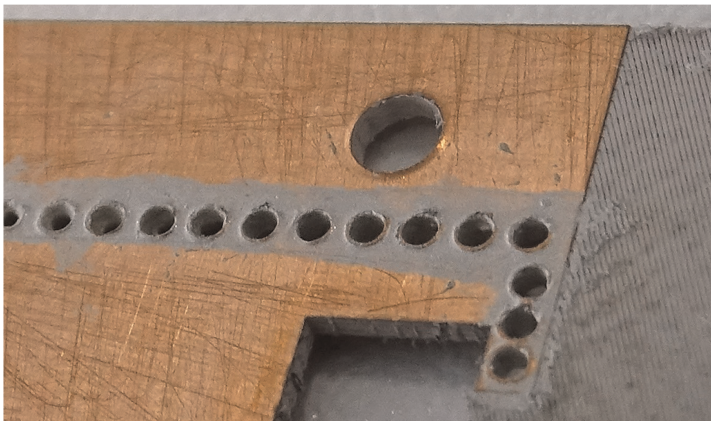
Figure 8. Through plated holes.
