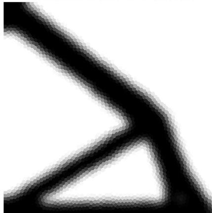
Figure 8: Example 2. Optimal topology computed with the proposed VEM formulation on an unstructured mesh with 2^6 elements along the thickness of the cantilever and filter radius r_{min} = 3.0d_m \approx 1.5/2^5 .
