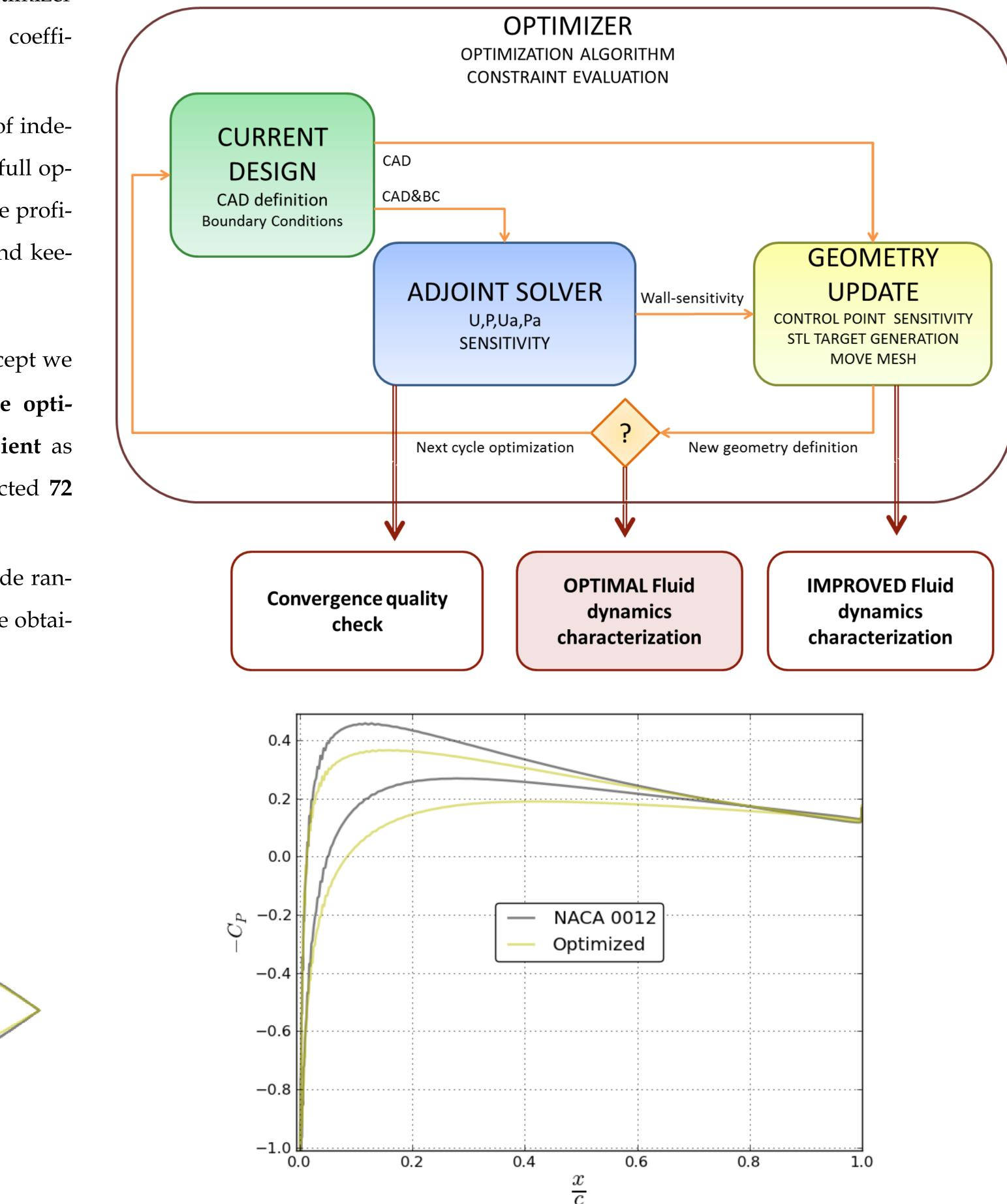
We tested several fluid dynamics conditions including a wide range of **Angles of Attack (AoA)** for the selected profile. All the obtained results were coherent, showing similar general patterns:
