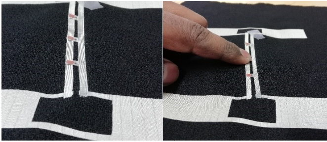
Fig. 6. In the Touch Prototype, all IC copper pads are initially separated from the electro-textile antennas (left); a specific IC can be “activated” by touching the copper pad, which will connect the IC to the antennas (right) and make the IC readable for the RFID reader.
