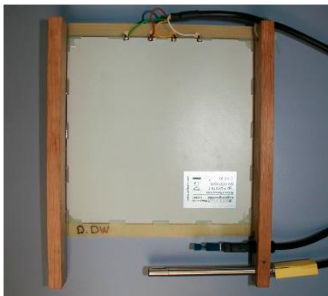
Figure 6. Auxiliary construction for fastening the thermal anemometer (shiny metallic probe at the bottom), the heat flow plate (gray square), and the combined air temperature and relative humidity sensors (black) into their relative positions indicated in the previous figures.
