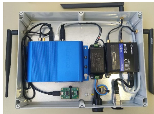
Figure 7: Gateway to use and control several sensor nodes
