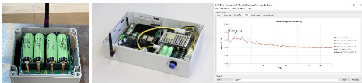
Figure 15: Sensor node with 3-axis acceleration sensor below the battery pack (left), HUB (center) and FFT analyses of the frequencies (right)
