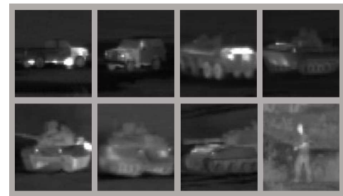
Figure 3: The manually created infrared (IR) dataset using video snapshots from the ATR database consists of eight classes, seven of them are civilian and combat vehicles and the last one is a human class.
