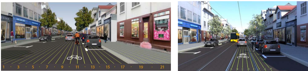
Figure 1. Left: Example of one of the trial images used in study 1 (condition pictogram without chevrons, with parking, person cycling ahead in 0.8 m distance from parked cars). Distance between the lines 0.04 m. Right: Example of one of the trial images used in study 2 (condition sharrows, with parking, with tram tracks, person cycling ahead in 0.6 m distance from parked car). Distance between the lines 0.03 m.
