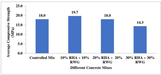
Fig. 4 - Average compressive strength of cubical specimen at 28 days (MPa)
