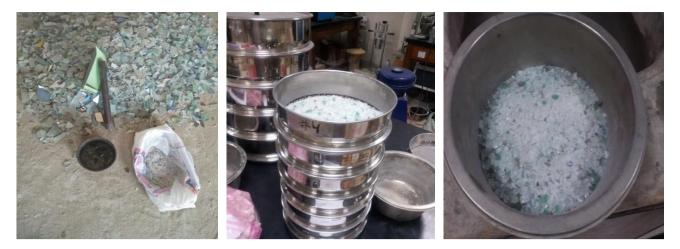
Fig. 1 - Preparation of Recycled Waste Glass (RWG)
