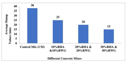
Fig. 3 - Average slump values of different concrete mixes
