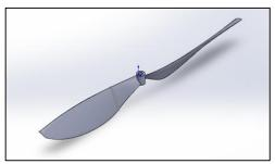
Fig. 3 - Propeller 3 with twisted blade
