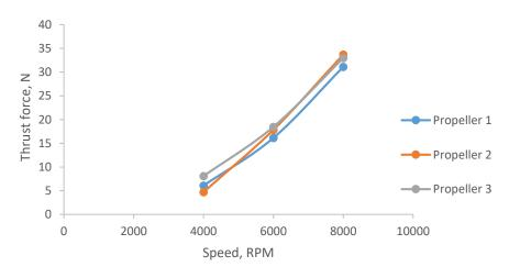
Fig. 8 - Comparison of thrust force on Propeller 1, 2 and 3
