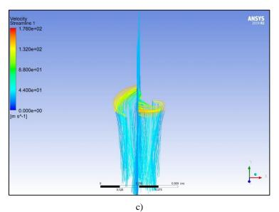
Fig. 12 - Velocity streamline of propeller 2 at speed (a) 4000 rpm; (b) 6000 rpm; (c) 8000 rpm
