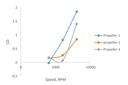
Fig. 10 - Graph speed, RPM against C<sub>D</sub> for all propeller
