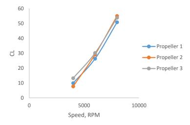
Fig. 9 - Graph speed, RPM against C<sub>L</sub> for all propeller
