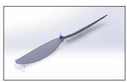
Fig.1 - Propeller 1 without twisted blade
