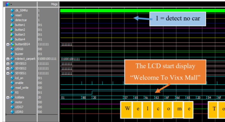
Fig. 7 - The timing diagram shows when no car is detected, the LCD a welcome message 'Welcome To Vixx Mall'
