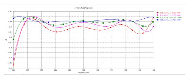
Fig. 5 - The insertion loss, (S21, dB) of circular waveguide with different twisting rates
