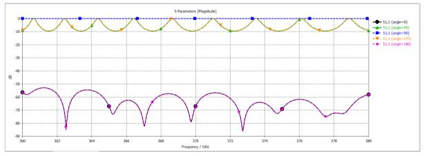
Fig. 2 - The return loss (S11, dB) at port 1 with different polarization angle, 0°, 45°, 90°, 135°, 180° at port 2 from 360 GHz to 380 GHz
