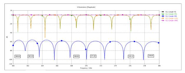
Fig. 3 - The insertion loss (S21, dB) with different polarization angle, 0°, 45 °, 90 °, 135 °, 180 ° at port 2 from 360 GHz to 380 GHz
