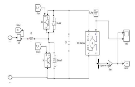
Fig. 8 - Motor and DC-DC converter system
