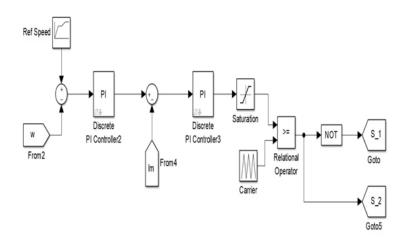
Fig. 9 - Motor PWM speed control
