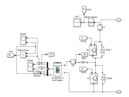
Fig. 6 - Battery and DC-DC converter system
