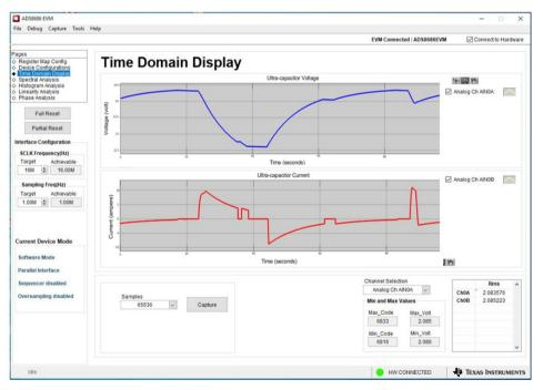
Fig. 18 - Voltage and current waveforms of ultracapacitor
