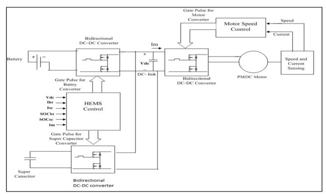
Fig. 4 - Block Diagram of Proposed HEMS system
