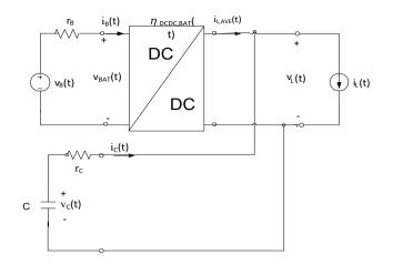
Fig. 2A - DC-DC converter connected with battery
