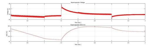
Fig. 15 - Supercapacitor voltage and SOC wave form
