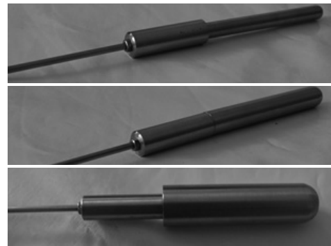
Fig. 5. Steel cathodes of increasing diameter.
