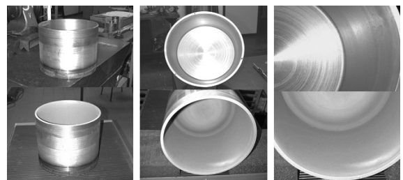
Fig. 6. Steel crucible before ( top ) and after ( bottom ) internal coating with alumina and silica by means of plasma spraying and plasma enhanced chemical vapour deposition.
