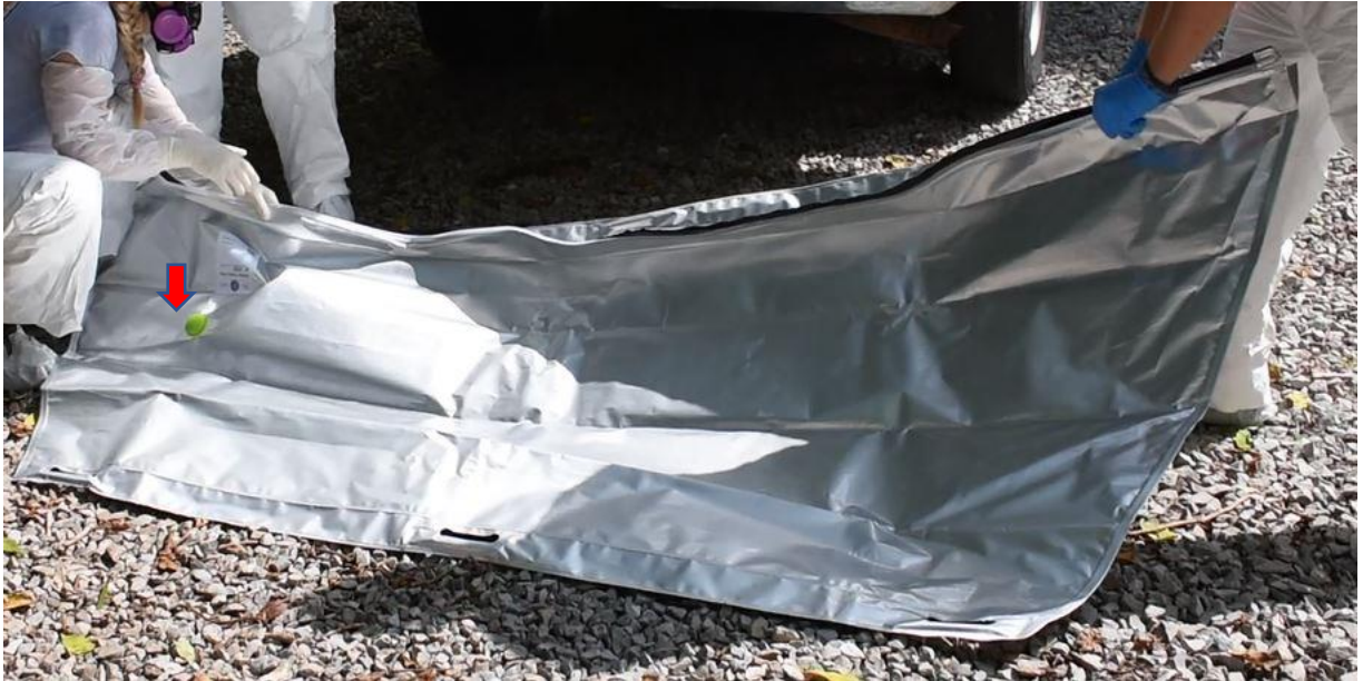
Figure 2.4 BBB prior to use. Observe the green valve pointed to by the red arrow. This is where the pump was attached to pump air out. The researchers are opening the seal. Observe the reflective coating here and how it reflects sunlight.
