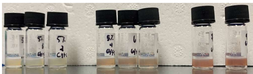
Figure 31. System 1C with cytochrome c in concentrations of 0.5 g/L (left group), 1.0 g/L (middle group), and 2.0 g/L (right group)
