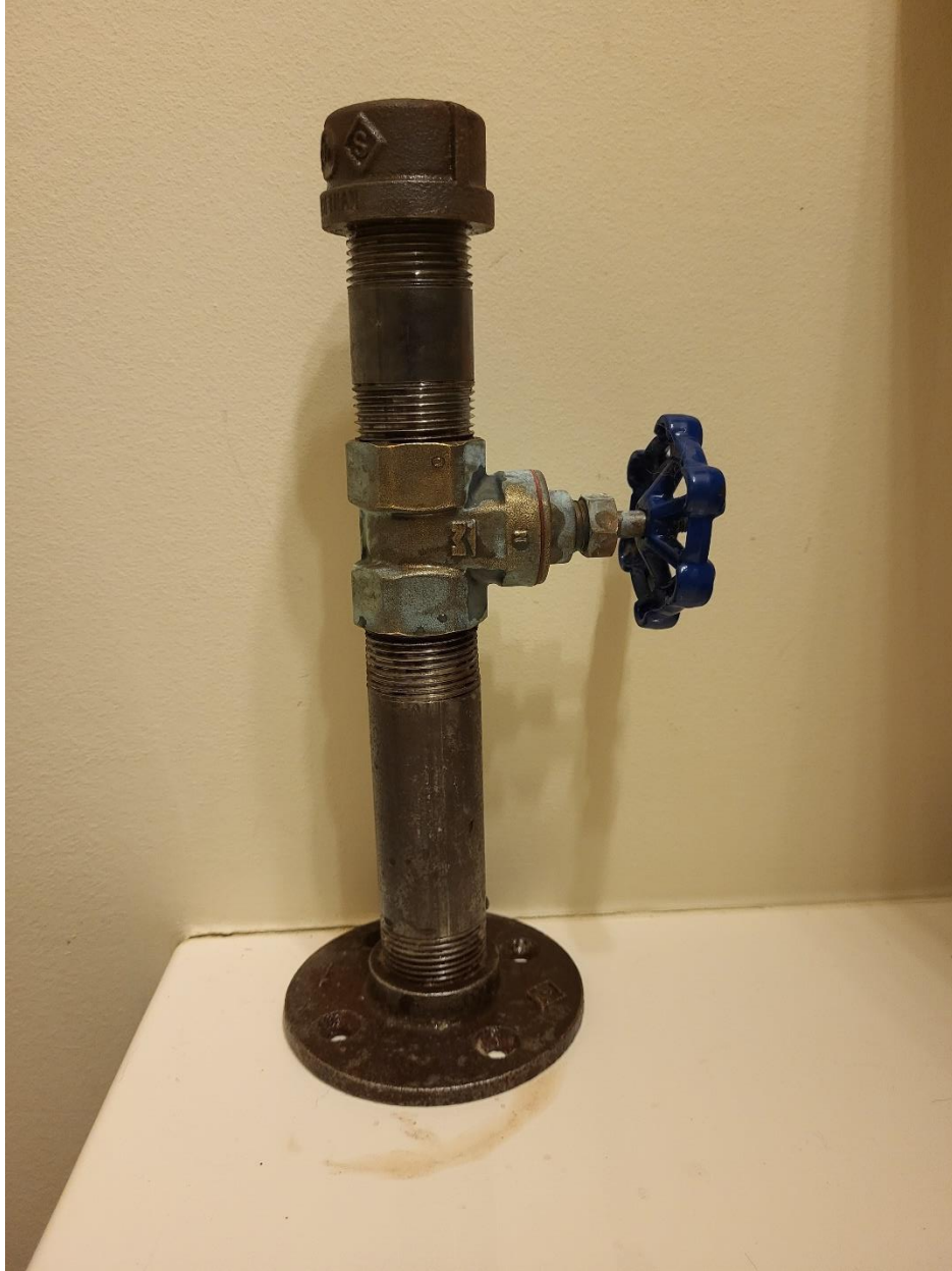
Figure 10 Improved SIU designed to prevent plastic contamination for use in small-scale density soil experiments
