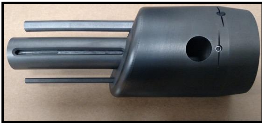
Figure 12. Triplet set of graphite collector probes inserted with MiMES for MRC 1
