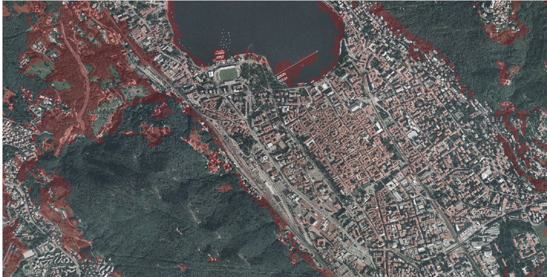
Figure 1 - Distribution of non-coherent pixels (red areas) in the Como municipality area for year 2010.
