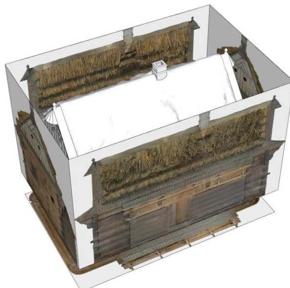
Fig. 7 – Orthogonal projections of textures onto the generalized model
