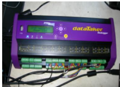
Fig. 6 - Data Taker Geologger data collecting system
