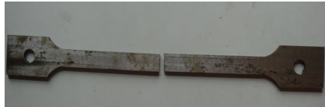
Fig. 3 - A steel plate with a gap at the mid-span
