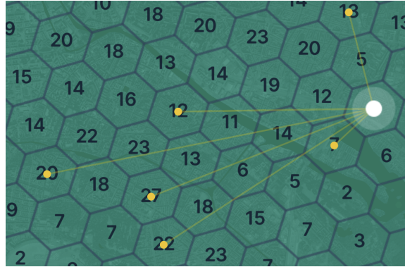
Figure 4.4: Helium Explorer representation of PoC challenge. The large white dot represents the Beaconer. Each of the yellow dots represents a witness. The background is a hexagonal grid depicting the number of hotspots in each hexagon. Figure is from [4].
