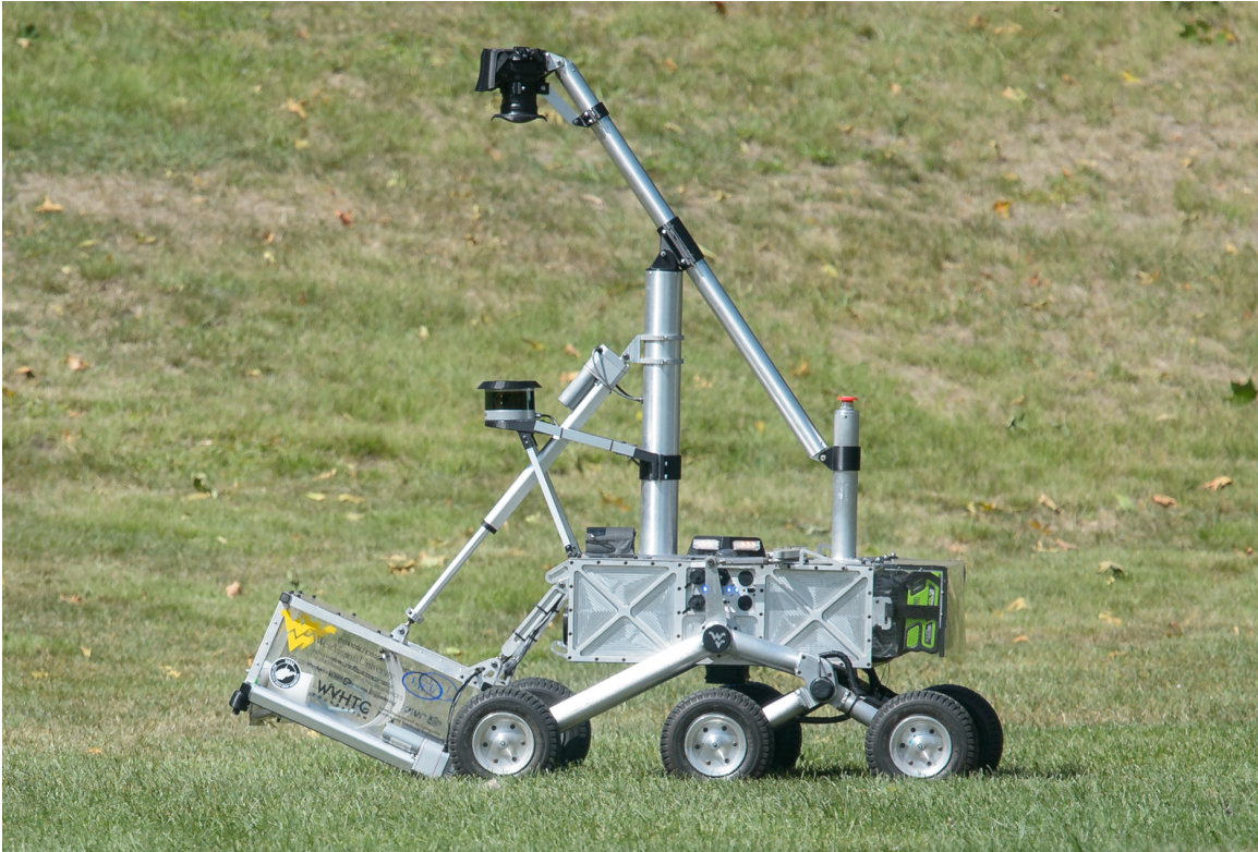
Figure 3.2.3: Cataglyphis picking up a sample during the NASA Sample Return Robot Centennial Challenge (photo credit: NASA/Joel Kowsky , © CC BY-NC-ND 2.0 )
