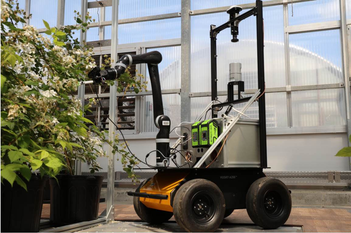
Figure 3.2.7: Precision pollination robot BrambleBee pollinating blackberry flowers in the WVU greenhouse
