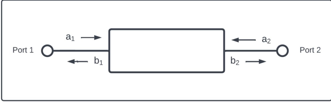
Figure 2: Single wave in a two-port electrical-element. Simple representation of a standard 2 port measurement for S-parameters.
