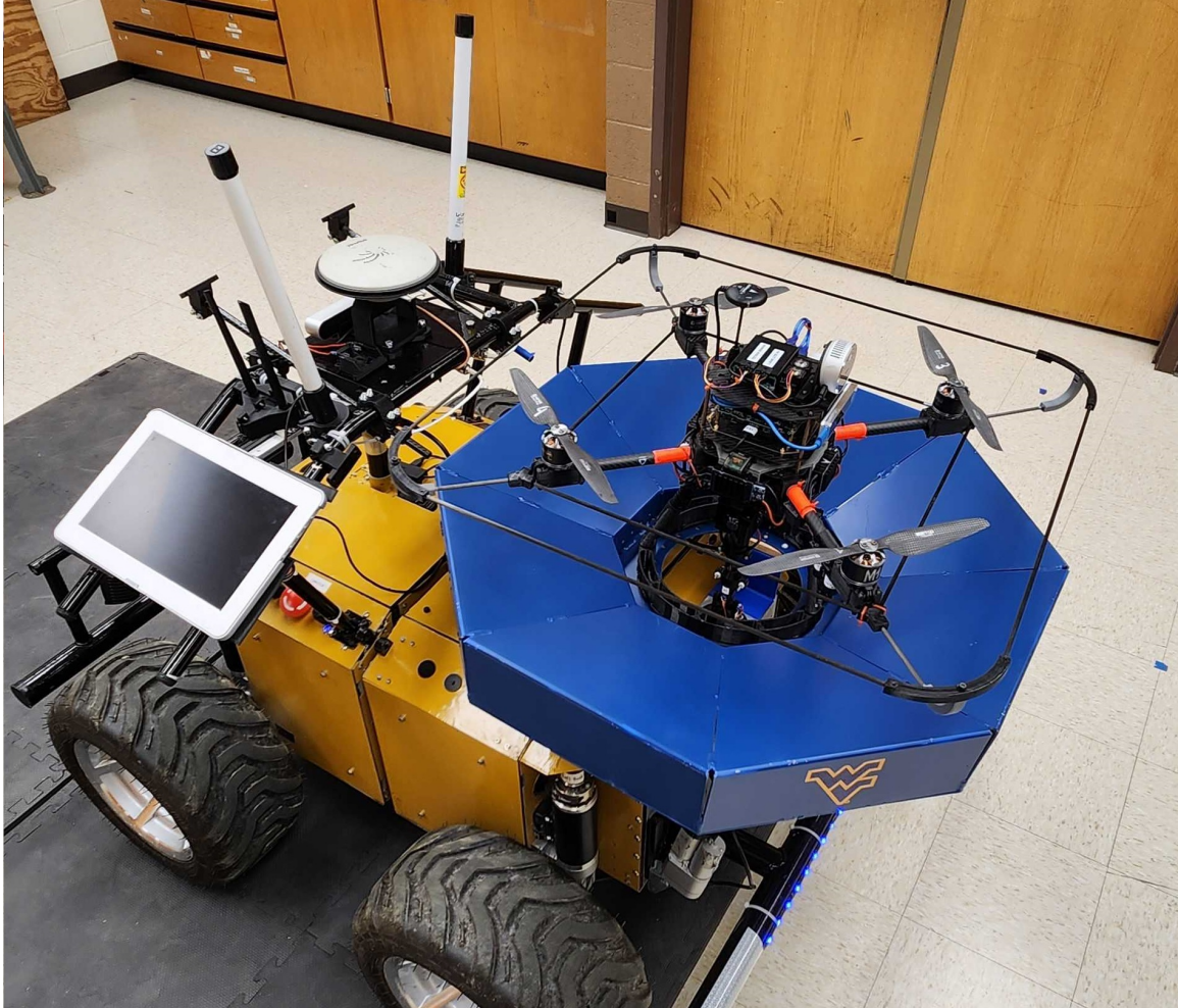
Figure 1.1: Ensemble of UGV and tethered UAV designed for stone mine mapping.
