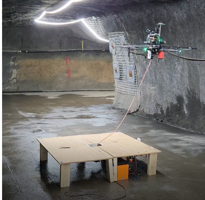
Figure 3.2: Image taken from testing of this project in NIOSH's experimental coal mining in Pittsburgh. This test was performed using a Matrice 100 UAV and a square wooden landing platform integrated with the tether angle sensor and winching mechanism.
