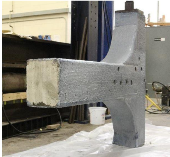
Figure 5.2 Specimen with a curve-shaped filler-module, coated with primer prior to the installation of FRP wraps. (Majjigapu 2020)
