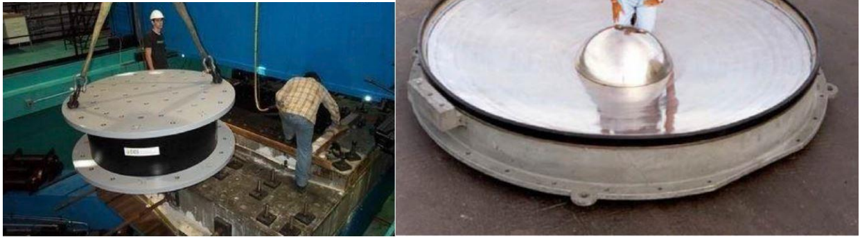
Figure 2.24 Left : Rubber bearing isolator with a diameter of 1300 mm, tested at the University of California, Berkeley (De Luca et al. 2019)
