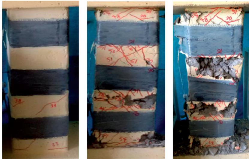
Figure 4.3 Damage and cracking patterns of specimen EBR2. (Kargaran and Kheyroddin 2019)
