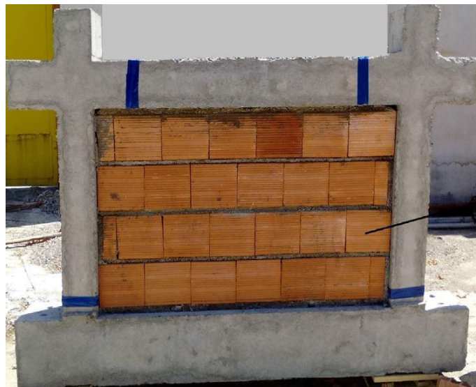
Figure 2.2 Masonry infill wall (Sharbatdar and Tajari 2021)
