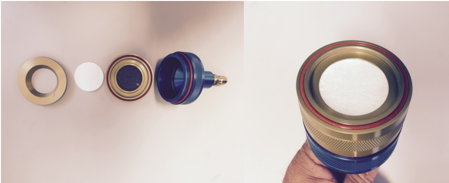
Air sample head and filter paper (below)
