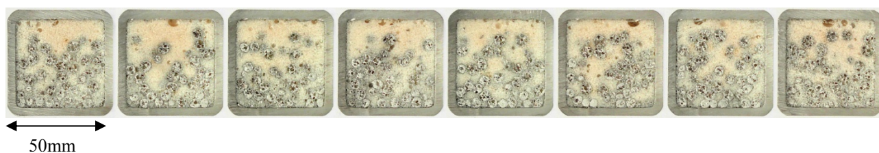
Figure 2. Aluminum foam filled tube cross sections.
